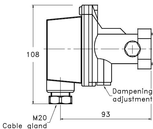
Switch point is approximately on the centreline of the instrument axis
